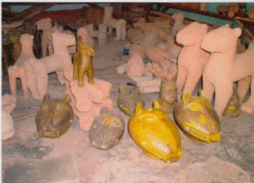
Fig. 6 Clay cores partly covered with wax for leopard figures and leopard heads in Benin style, ready to be finished in the storage of a caster at the rue d'Artisanat in Fumban 2004. Photo: Barbara Plankensteiner.
